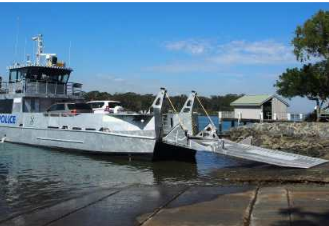
Queensland Water Police PV Stewart Kerlin ii Built BY Norman Wright BOATBUILDERS at RIVERGATE Nyalic Applied over a sanded and washed surface. NO ACID USED
